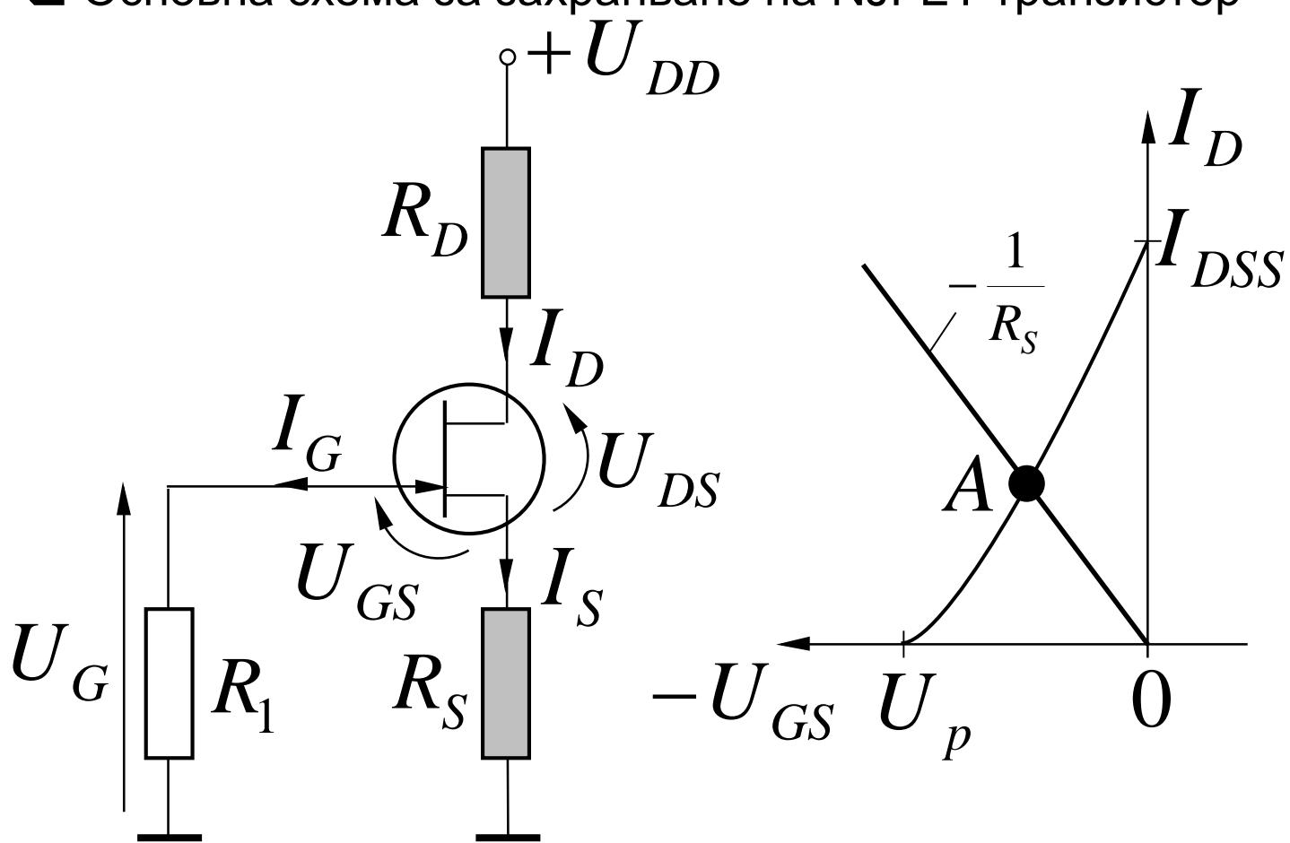
$$I_D = -\frac{1}{R_D + R_S} (U_{DS} - U_{DD}) ;$$
