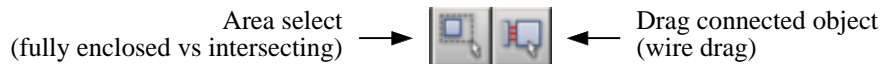
Figure 29. Buttons on the toolbar in Capture for controlling the way in which objects are selected and whether wires are reconnected when an object is moved.
