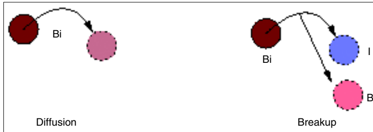
Figure 33 Impurity pairs can diffuse or break up into a substitutional plus an interstitial or a vacancy
