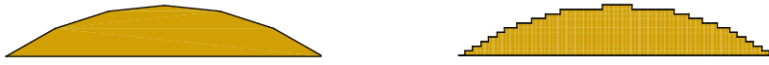
Figure 22 (Left) Actual curve region in the geometry and (right) corresponding approximation of this region in tensor mesh
