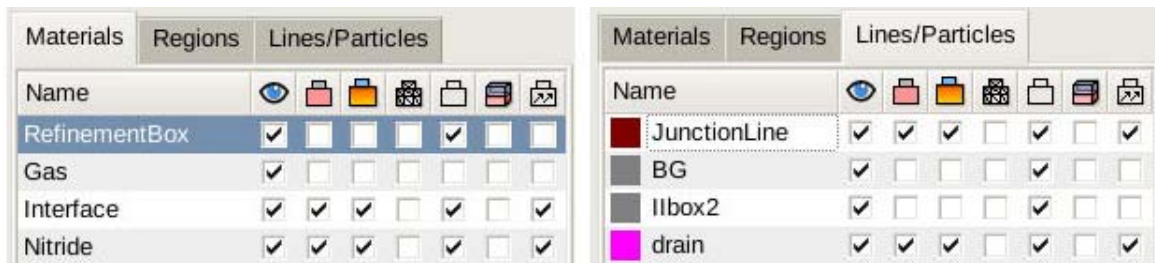
Figure 32 (Left) Materials tab showing RefinementBox and (right) Lines/Particles tab showing refinement boxes
