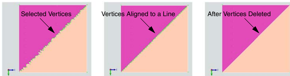
Figure 23 Two-dimensional boundary simplification, align to line, and vertex removal
