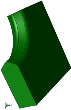
Figure 53 Corner sweeping around an axis; the initial profile is the same as in Figure 52
