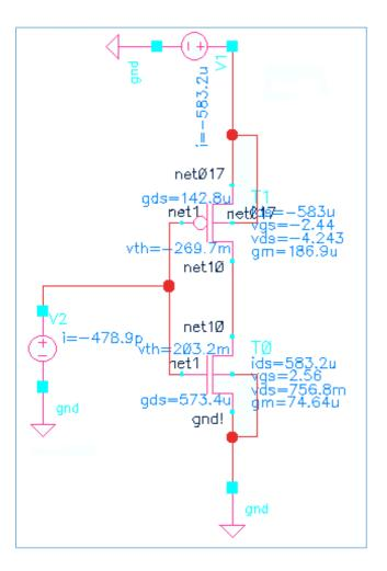
In the process of technology development the first revision of the models is based on TCAD simulations or models from previously developed technology nodes. As the technology development advances the TCAD data is substituted by measurement data.
