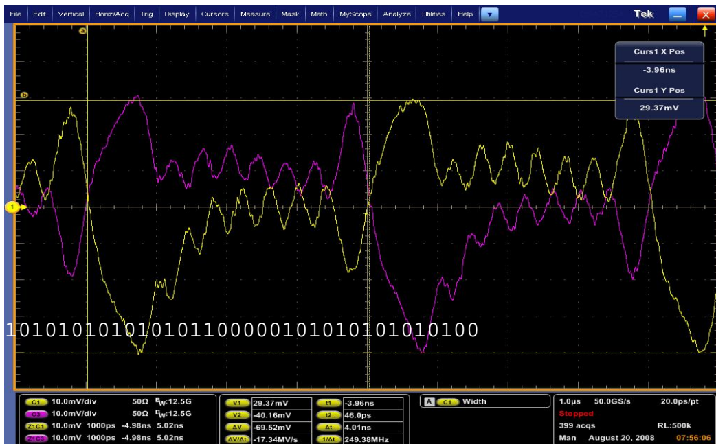
Figure 3. Received signal at the input to receiver at the end of a lossy transmission line
