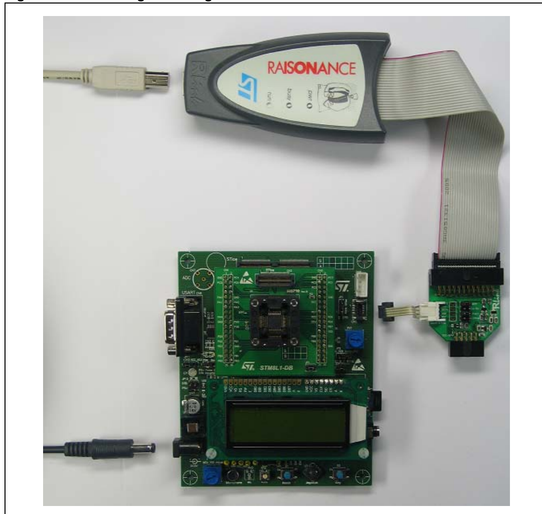
Figure 22. Connecting the debug instrument to the STM8L101-EVAL evaluation board
