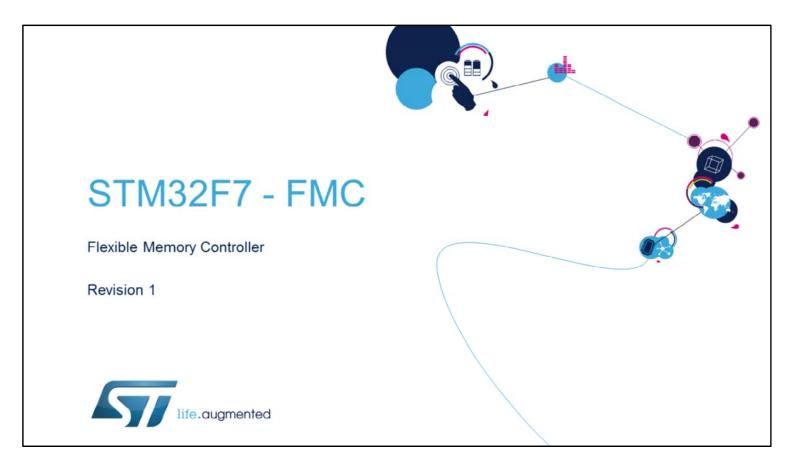
Hello, and welcome to this presentation of the STM32F7 Flexible Memory Controller. It covers all the features of this interface which is used to connect external memories such as NOR Flash, NAND Flash, SRAM, PSRAM and SDRAM.
