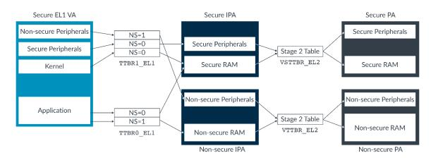
Unlike the Stage 1 tables, there is no NS bit in the Stage 2 table entries. For a given IPA space, all the translations either result in a Secure or Non-secure physical address, which is controlled by a register bit. Typically, the Non-secure IPAs translate to Non-secure PAs and the Secure IPAs translate to Secure PAs.
