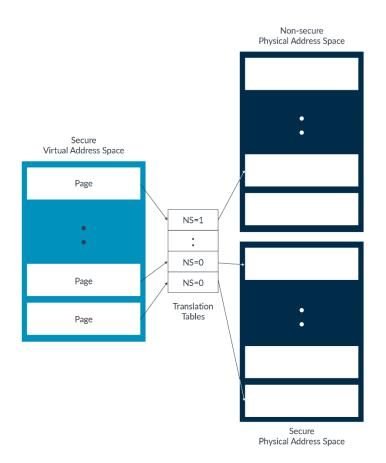
Note: In Secure state, when the Stage 1 MMU is disabled all addresses are treated as Secure.
