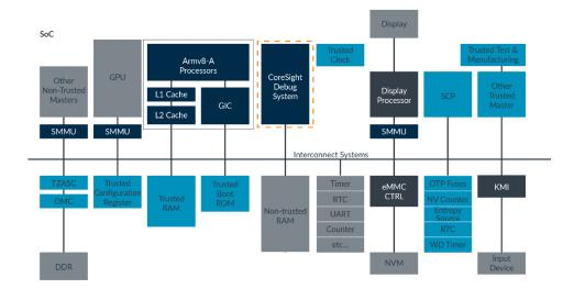
Modern Arm systems include extensive features to supporting debugging and profiling. With TrustZone, we must ensure that these features cannot be used to compromise the security of the system.
