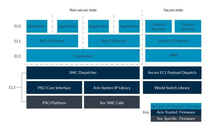
The SMC dispatcher handles incoming SMCs. The SMC dispatcher identifies which SMCs should be dealt with at EL3, by Trusted Firmware, and which SMCs should be forwarded the Trusted Execution Environment.
