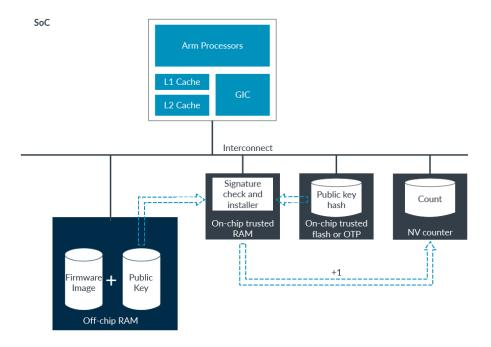
The downloading of the image is carried out in Non-secure state. The image itself is a not a secret, so we do not protect its confidentiality. The downloaded image is placed in memory and a request is issued to Secure state to install it.
