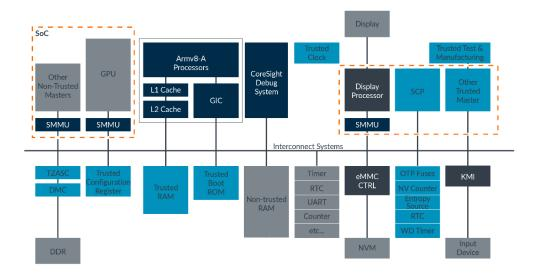
The A-profile processors in the system are TrustZone aware and send the correct security status with each bus access. However, most modern SoCs also contain non-processor bus masters, for example, GPUs and DMA controllers.
