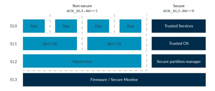
Note: Support for Secure EL2 was first introduced in Armv8.4-A and support remains optional in Armv8-A.
