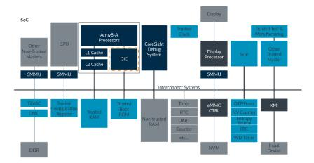
The Generic Interrupt Controller (GIC), supports TrustZone. Each interrupt source, called an INTID in the GIC specification, is assigned to one of three Groups:
