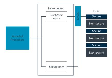
The TZASC is similar to a Memory Protection Unit (MPU), and allows the address space of a device to split into several regions. With each region specified as Secure or Non-secure. The registers to control the TZASC are Secure access only, permitting only Secure software to partition memory.
