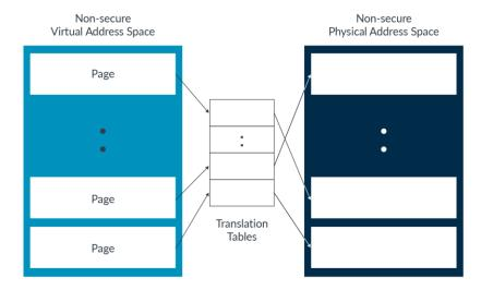
While in Secure state, software can access both the Secure and Non-secure physical address spaces. The NS bit in the translation table entries controls which physical address space a block or page of virtual memory translates to, as shown in the following diagram:
