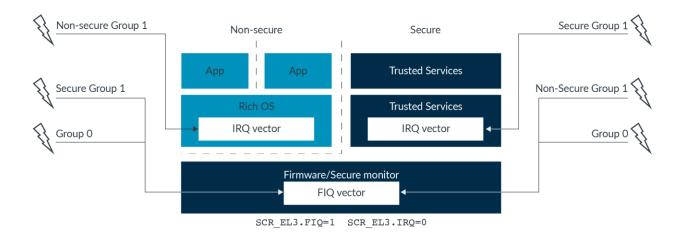
The preceding diagram shows one possible configuration. Another option that is commonly seen is for FIQs to be routed to EL1 while in Secure state. The Trusted OS treats the FIQ as a request to yield to either the firmware or to Non-secure state. This approach to routing interrupts gives the Trusted OS the opportunity to be exited in a controlled manor.
