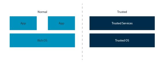
The Normal world runs a rich software stack. This software stack typically includes a large application set, a complex operating system like Linux, and possibly a hypervisor. Such software stacks are large and complex. While efforts can be made to secure them, the size of the attack surface means that they are more vulnerable to attack.
