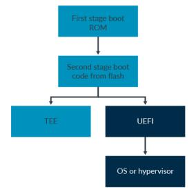
In our example, the first code that runs is the boot ROM. We must implicitly trust the boot ROM, because there are no earlier stages of boot to verify its contents. Being in ROM protects the initial boot code from being rewritten. Keeping the initial boot code on-chip prevents it from being replaced, so we can implicitly trust it. The boot ROM code is typically small and simple. Its main function is to load and verify the second stage boot code from flash.
