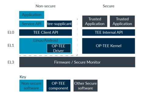
The OP-TEE kernel runs in S.EL1, hosting Trusted applications in S.EL0. The Trusted applications communicate with the OP-TEE kernel through the TEE Internal API. The TEE Internal API is a standard API developed by the GlobalPlatform group. GlobalPlatform work to develop standard APIs, which are supported by many different TEEs, not just OP-TEE.
