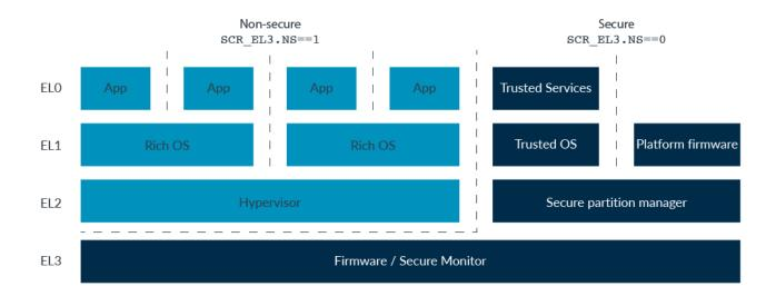
Rather than a full hypervisor, S.EL2 typically hosts a Secure Partition Manager (SPM). An SPM allows the creation of the isolated partitions, which are unable to see the resources of other partitions. A system could have multiple partitions containing Trusted kernels and their Trusted services.
