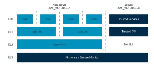
As previously described in **Switching between Security States**, EL3 is used to host firmware and the Secure Monitor. Secure EL0/1 host the Trusted Execution Environment (TEE), which is made up of the Trusted services and kernel.
