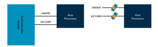
By blowing fuses during manufacture, external debug can be permanently disabled. Using fuses does make in-field debug more difficult. When the fuses are blown, they cannot be unblown. An authentication module is more flexible.
