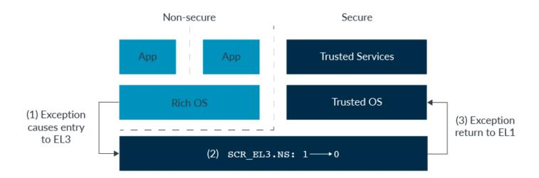
The preceding diagram shows an example sequence of the steps that are involved in moving between Security states. Taking these one step at a time:
