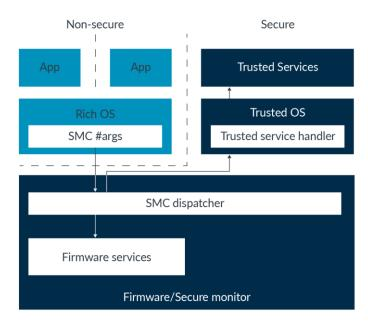
In a bid to standardize interfaces, Arm provides the SMC Calling Convention (DEN0028) and Power State Coordination Interface specification (DEN0022). These specifications lay out how SMCs are used to request services.
